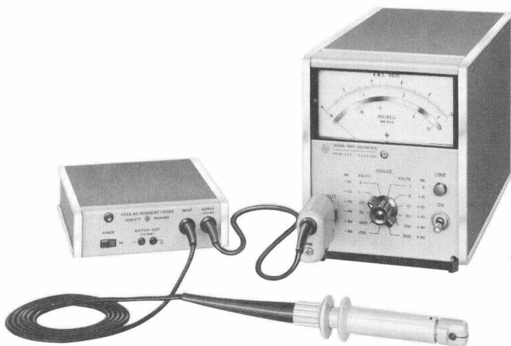
Fig. 6. RMS values of alternating currents are measured with combination of -hp- Models 456A Current Probe and 3400A RMS Voltmeter. Current Probe sensitivity of 1 mv/1 ma permits voltmeter scales to be read directly as current.
